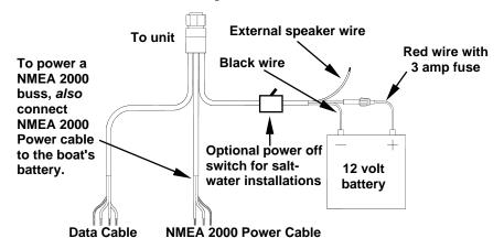
Power connections for LCX-17M sonar/GPS unit.
